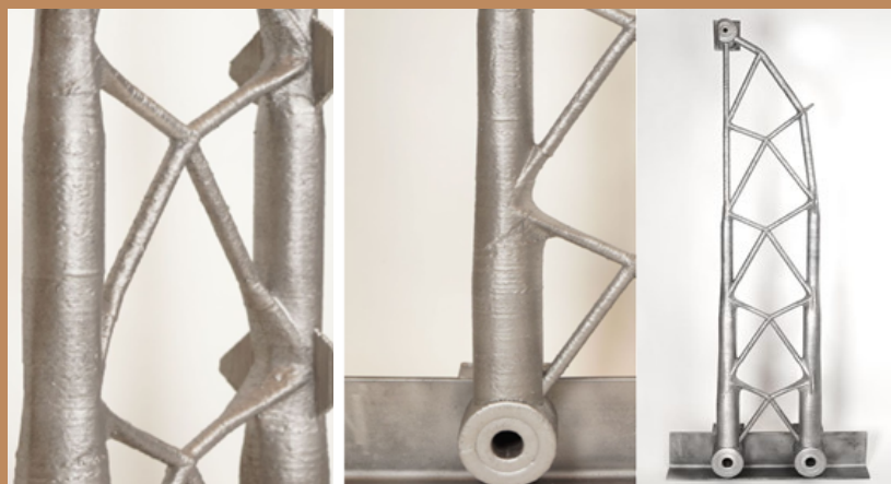
INTEGRADDE truss in M1 Metal AM System - MX3D
