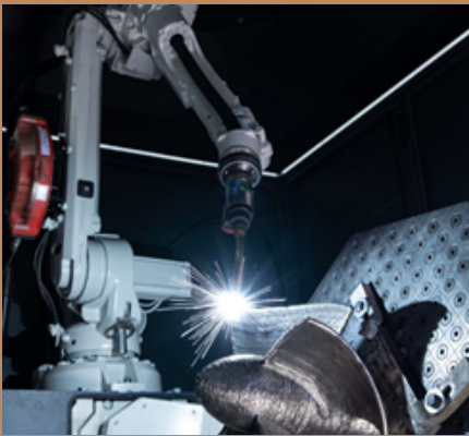
Robotic WAAM by M1 Metal AM System
