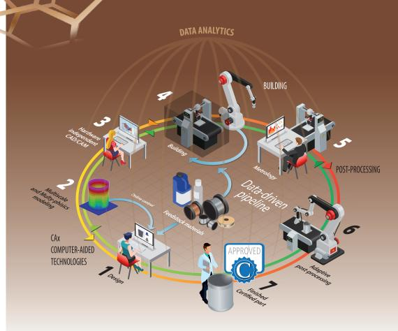
Intelligent data-driven pipeline for the manufacturing of certified metal parts through Direct Energy Deposition process
