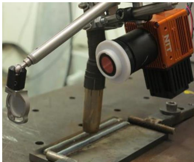
Figure 3.- Set up used at West University for monitoring WAAM processes
